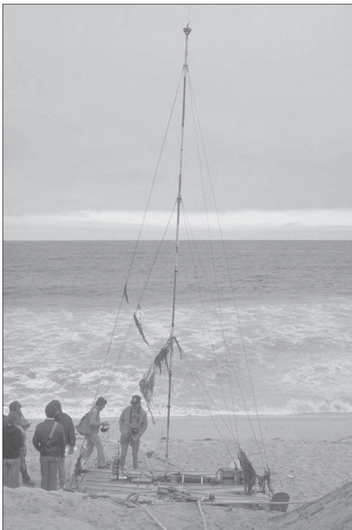
Figure 8.3 Photograph of the sled used by Sallenger et al. (1983) to measure wave and current dynamics and topography on the California coast. The sled was winched offshore as well as onshore, necessitating a complicated offshore mooring and providing a number of logistical difficulties. Other systems use a boat to carry the sled offshore and only winch it onshore.
