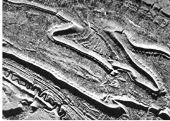
Syncline structures (in Pennsylvania) on SAR imagery
