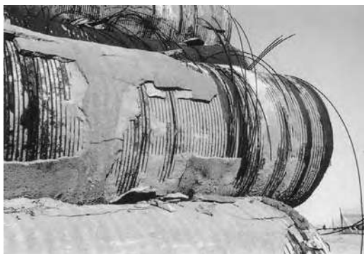
Plate 106 Damaged water pipelines in central Namibia. They proved to be unable to withstand the corrosive conditions associated with the foggy, salty environment of the Namib, and had to be replaced after only a few years in service
